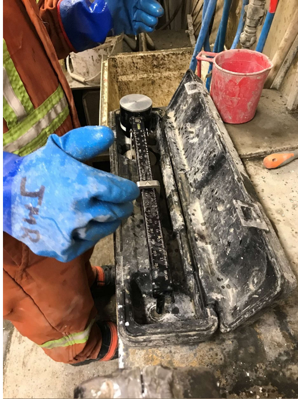
Checking grout density
