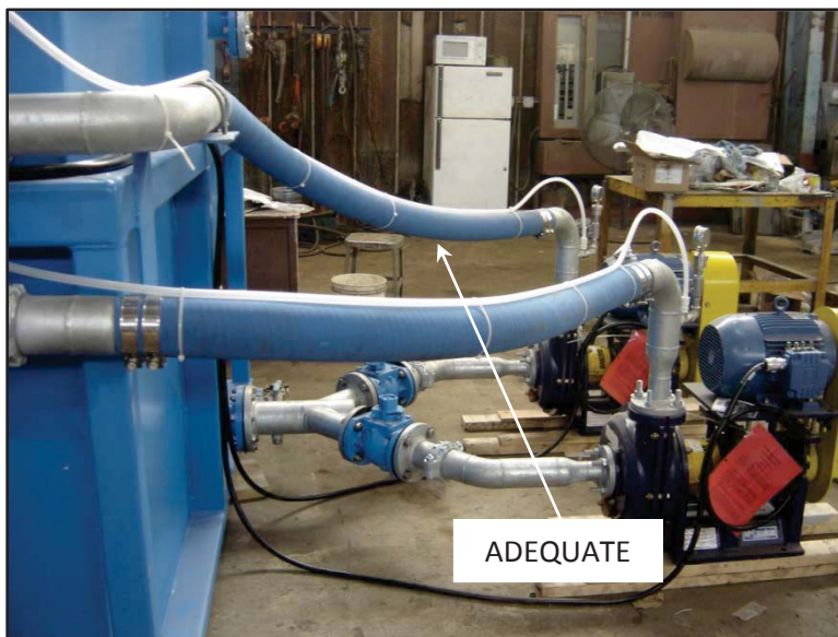
MICROSAND RECIRCULATION PUMP ADEQUATE HOSE INSTALLATION
