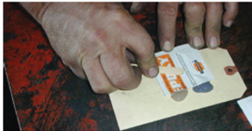
2. Extrude epoxy from package & mix thoroughly
