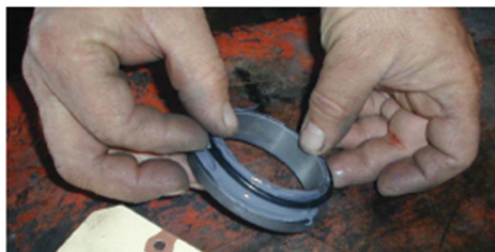
4. Place 'O' Ring (D10) on outer rim of Hard Wear Face (D11). Position 'O' Ring at leading edge.
