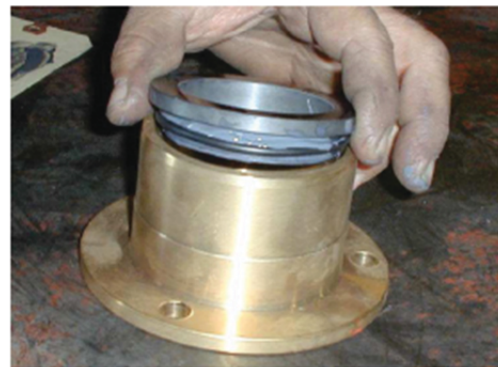
5. Position Hard Wear Face & 'O' Ring into Gland Adjuster (D03U)
