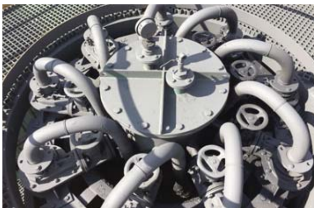
Image: PVEG50M manual polyamide body pinch valves in a hydrocyclone at Kara Mine, TMM, Tasmania, Australia.
