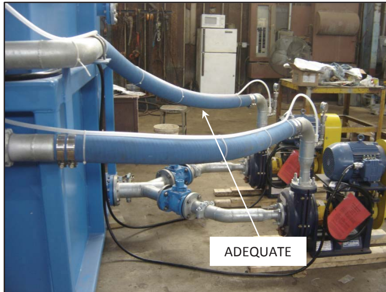
MICROSAND RECIRCULATION PUMP ADEQUATE HOSE INSTALLATION
