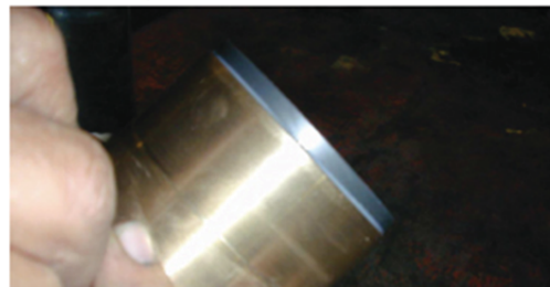
7. Wipe off excess epoxy
