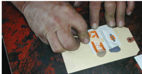
2. Extrude epoxy from package & mix thoroughly
