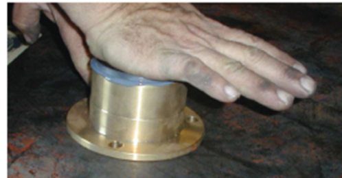
6. Using a slight twisting motion Carefully push Hard Wear Face into Adjuster
