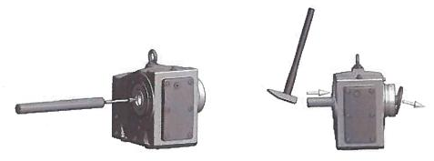
Figure 8: Removing the factory-fitted closing cap
