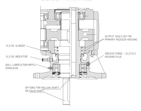
VL2 & VL3 greased bearing lubrication Standard factory lube:
