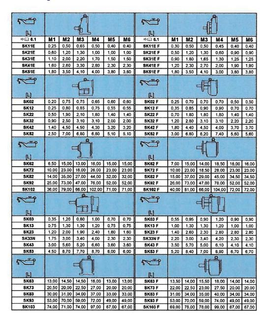
Table 7: Lubricant quantities for helical gear units
