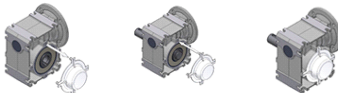
Fig. 16: Removal and fitting of the cover cap
