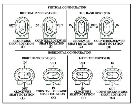
FIGURE 2-1 - BLOWER MOUNTING CONFIGURATIONS
