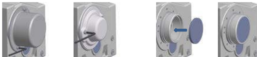
Figure 15: Fitting the covers, Option SH, Option H, and Option H66
