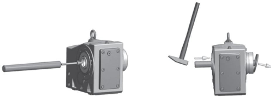
Figure 8: Removing the factory-fitted closing cap
