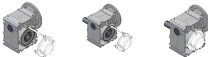
Fig. 16: Removal and fitting of the cover cap
