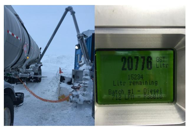
Photo 3: Agnico Eagle Ltd.'s Refueling Station – Loading arm and Scully System
