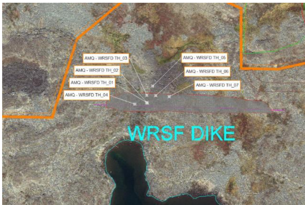
Figure 4: WRSF Thermistor locations
