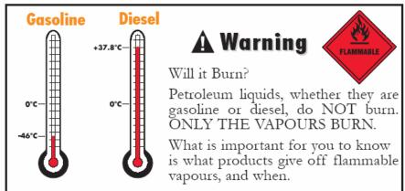
Different petroleum liquids give off flammable vapours at different temperatures (this is called flash point). The thermometers above show when gasoline (-46°C) and diesel (+37.8°C) give off flammable vapours.
