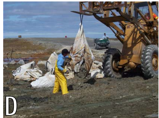
Photographs C & D: Picture C showing a mega bag lifted by the front loader, while picture D showing the bag sliced open to let the drilling cuttings out of the bag.
