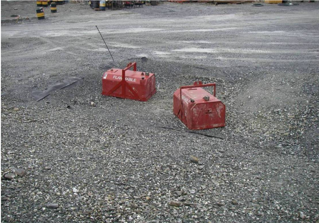
Photo 15: Tidy tanks refueling area in lined facility.
