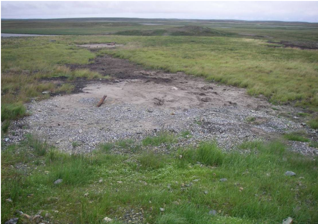
Photo 41: Example of permafrost degradation at the historic drill site. Note: same gravel (crushed ore) has been placed at one time in an attempt to mitigate the damage.
