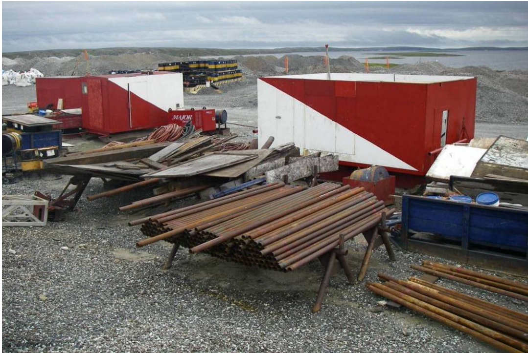
Photo 14: Drill supplies in foreground and jet fuel stored in drums on pallets in the background. No secondary containment.
