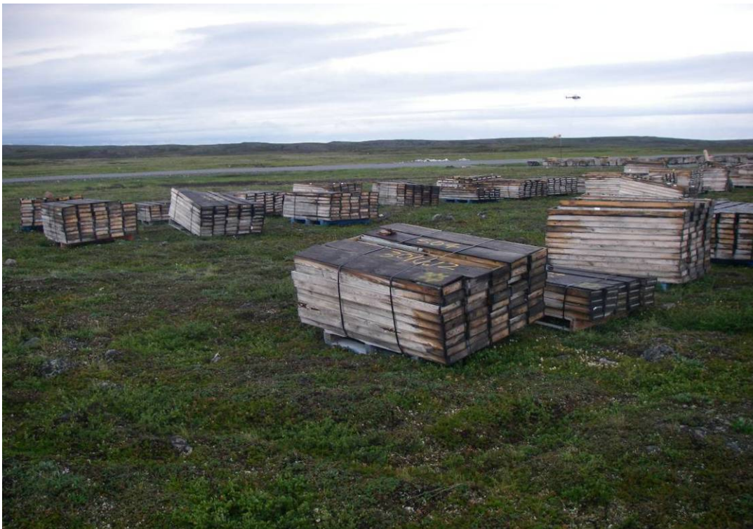
Photo 38: Core storage area. Many of the pallets are stored directly on the tundra.
