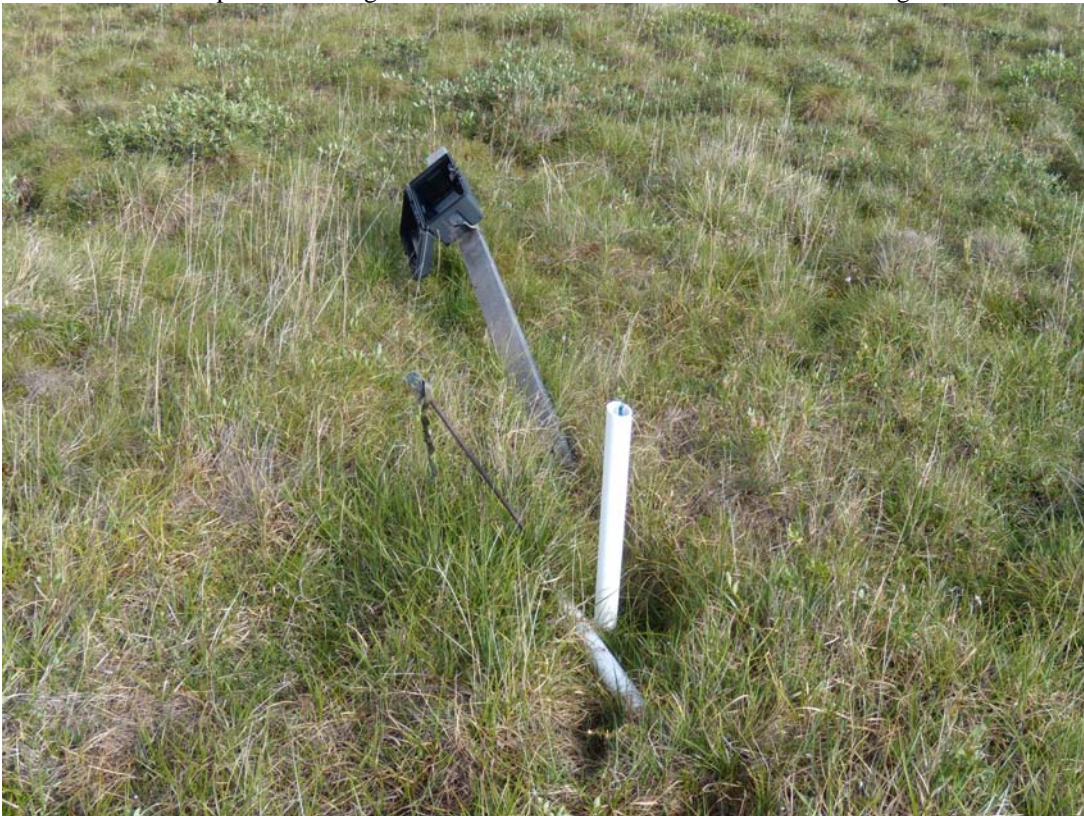
Photo 56: Drill hole 12259-03 (BH3) with thermistor string #1049. The cable has been severed.
