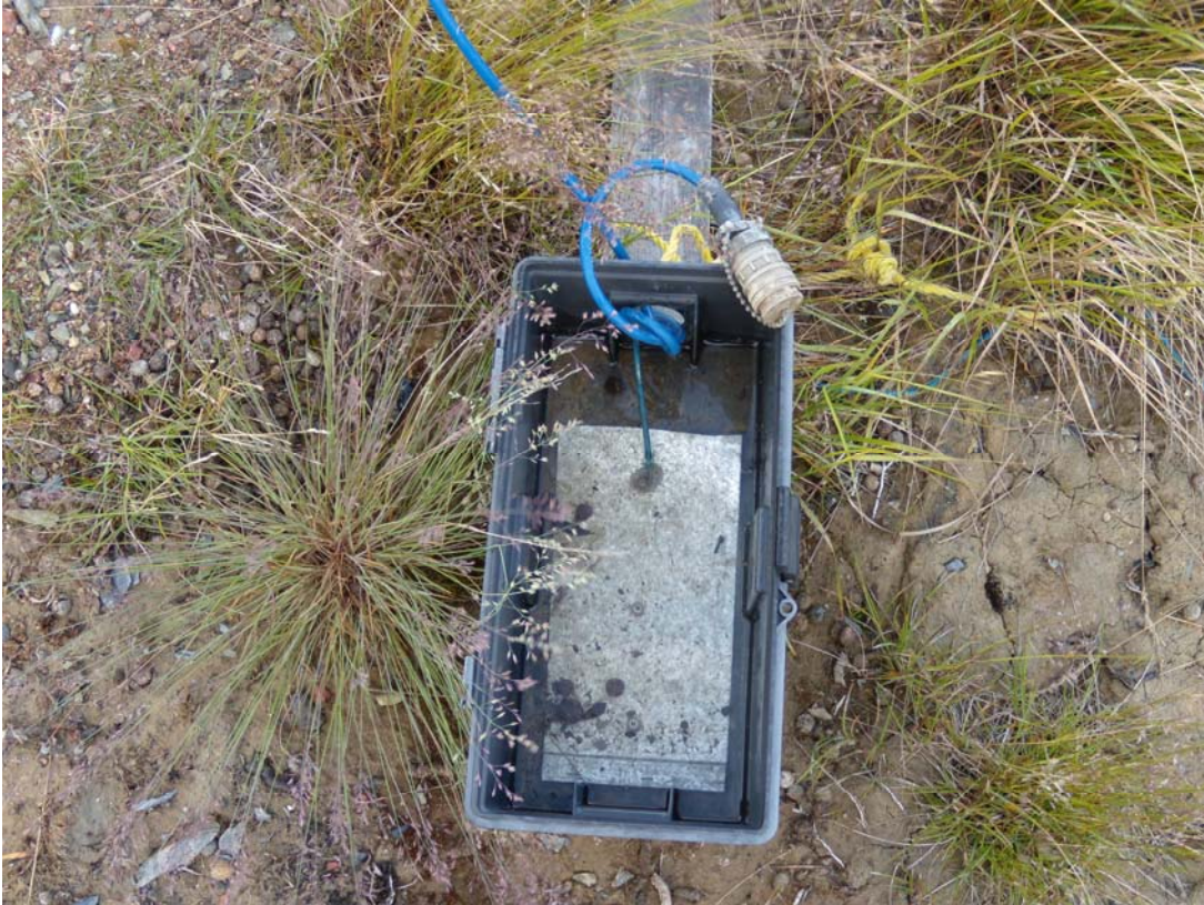
Photo 61: Close-up of the readout box and terminal connector for the thermistor string on drill hole 97NOD176.
