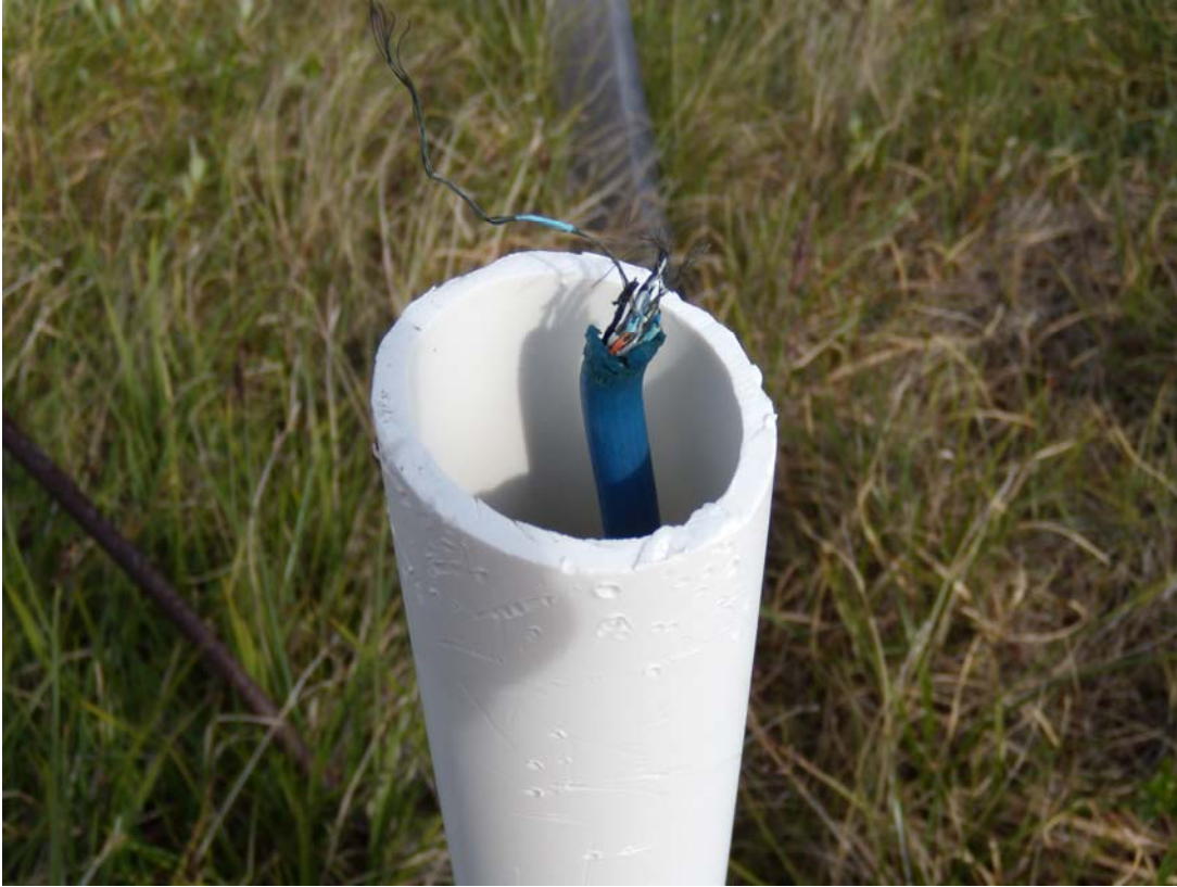
Photo 57: Close-up of the severed cable on drill hole 12259-03 (BH3) with thermistor string #1049.
