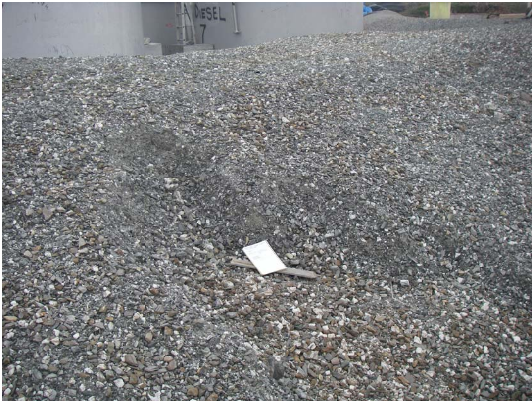
Photo 30: Evidence of small sloughing failures on the northern outside berm of the fuel tank farm. These failures do not pose a risk to the containment design at this time.
