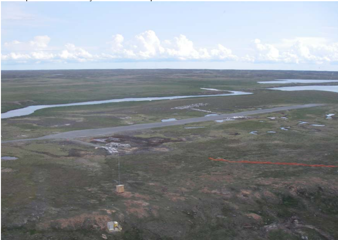
Photo 4: Oblique aerial view of the Boston airstrip looking south-east. Note the permafrost degradation damage visible at the north-west end of the airstrip.
