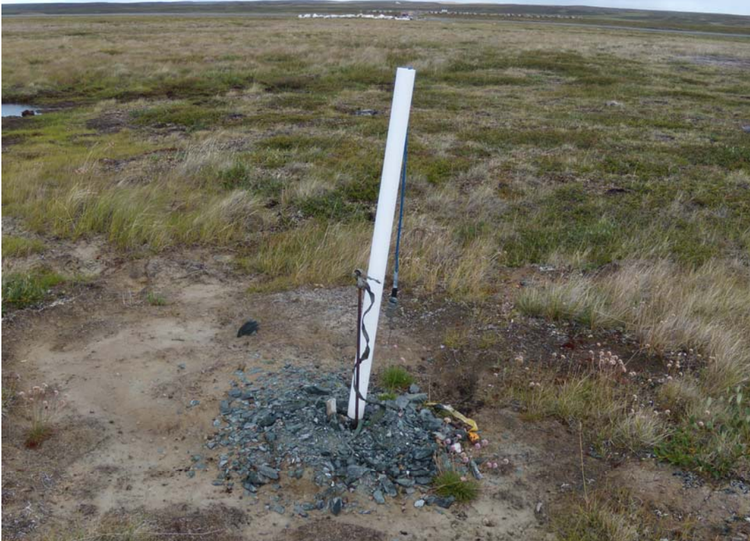
Photo 58: Drill hole 12259-05 (BH5) with thermistor string #1050.
