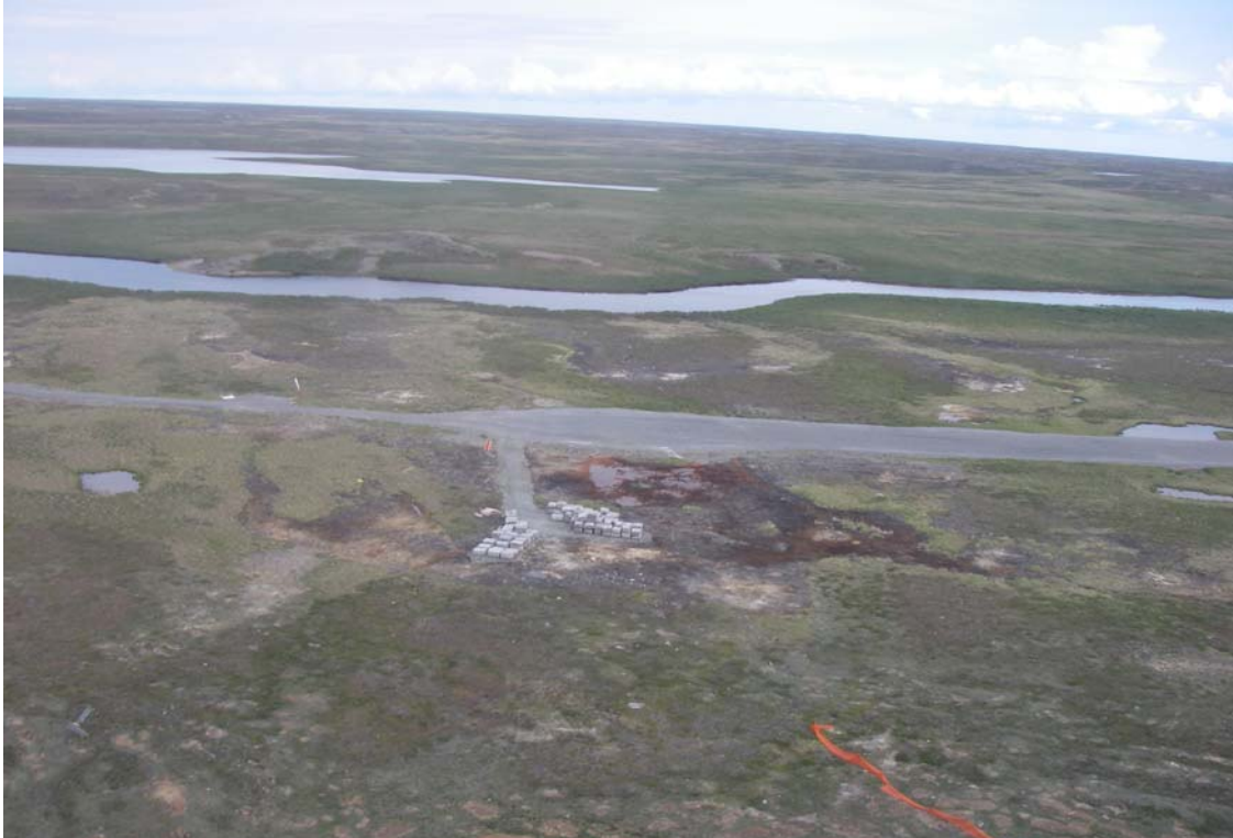
Photo 5: Oblique aerial view of the northern end of the Boston airstrip looking east. The brown patch between the airstrip and the core storage road (north airstrip core storage area) is an area of vegetation dieback and permafrost damage.
