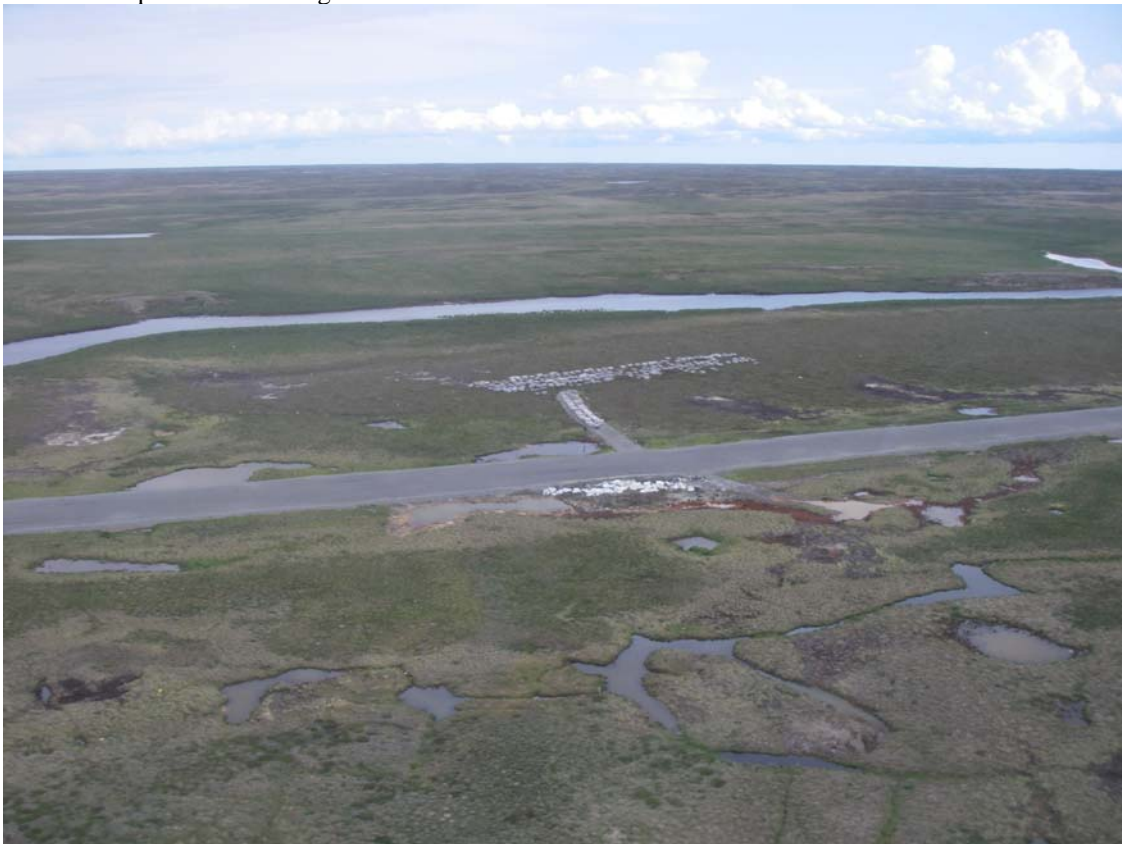
Photo 6: Oblique aerial view of the central section of the Boston airstrip looking east. The east airstrip core storage area is shown in the background. Permafrost damage is shown immediately west of the airstrip in the center of the photo.
