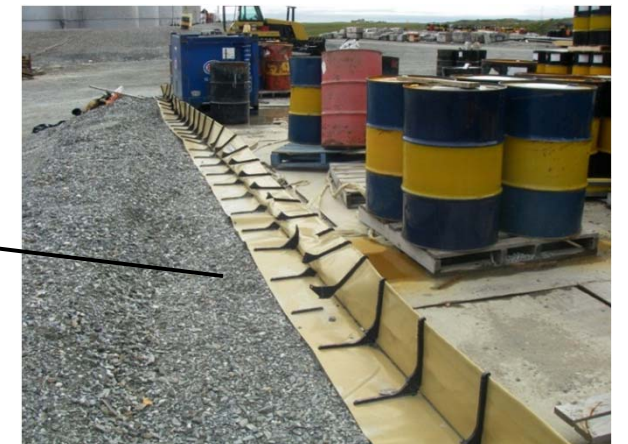
Containment berm collapsed and in need of repair.
