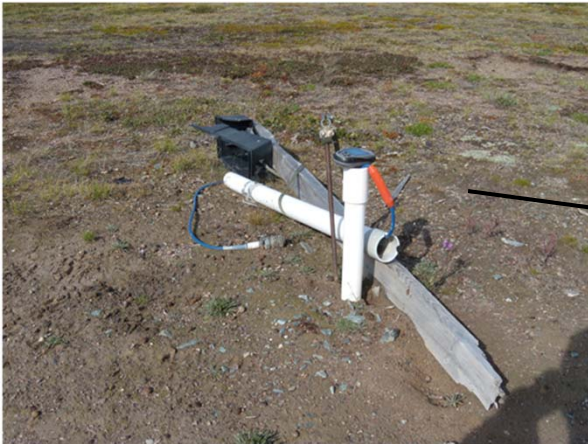
Drill hole 12259-06 (BH6) with thermistor string #1051.
