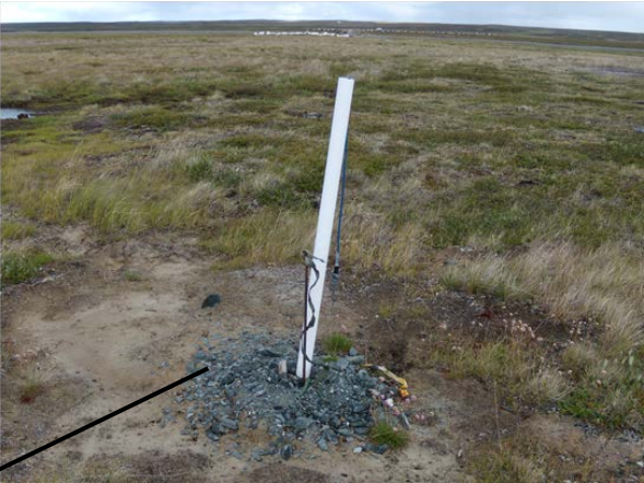
Drill hole 12259-05 (BH5) with thermistor string #1050.
