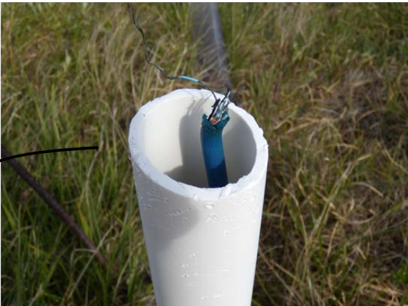
Close-up of the severed cable on drill hole 12259-03 (BH3) with thermistor string #1049.
