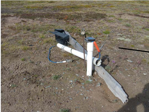
Drill hole 12259-06 (BH6) with thermistor string #1051.
