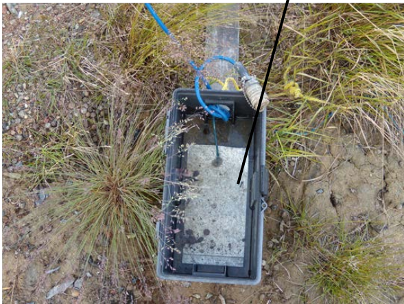
Close-up of the readout box and terminal connector for the thermistor string on drill hole 97NOD176.
