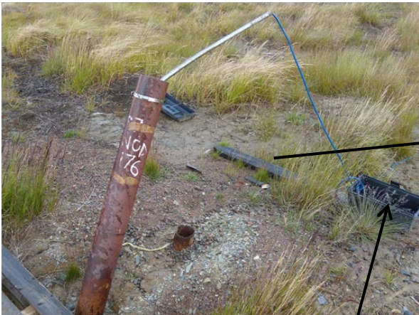
Drill hole 97NOD176 with thermistor string.
