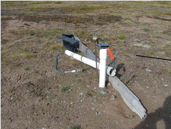
Drill hole 12259-06 (BH6) with thermistor string #1051.
