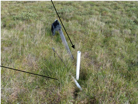
Drill hole 12259-03 (BH3) with thermistor string #1049. The cable has been severed.
