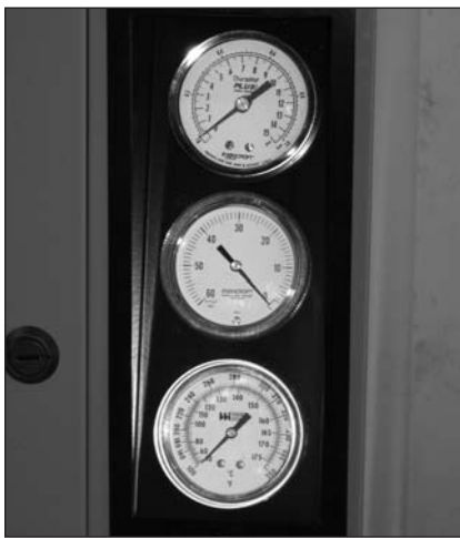
Discharge pressure, filter restriction, and temperature gauges are standard.
