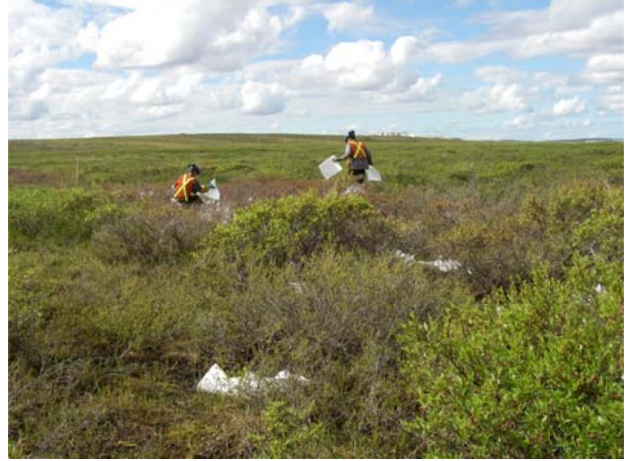
July 14, 2011. View north toward Boston Camp, downhill from Orbit 25 Drill Rig. Crew placing absorbent pads on standing pools to absorb residual hydrocarbons, if present.
