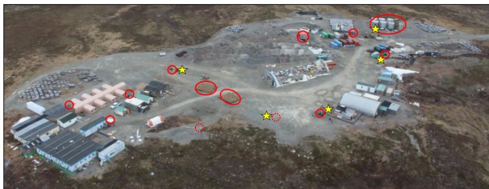
Plate D.1. Boston Camp (Note: Red circles are fuel or chemical storage locations, smaller storage locations may vary. Yellow star indicates spill kit locations.)
