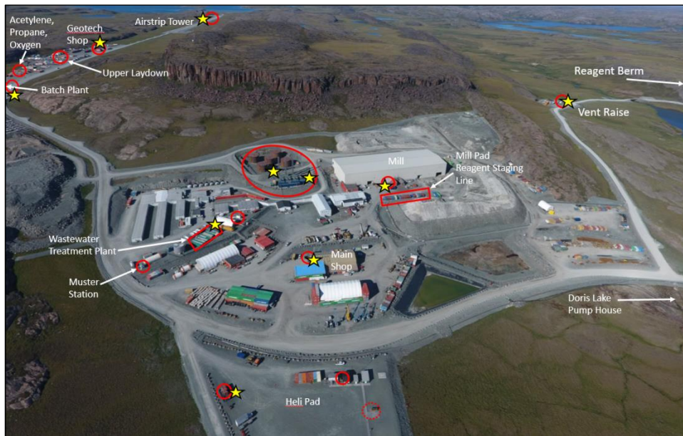
Plate A.2. Doris Camp (Note: Red circles are fuel or chemical storage locations, smaller containment locations may vary. Yellow stars indicate default spill kit locations.)
