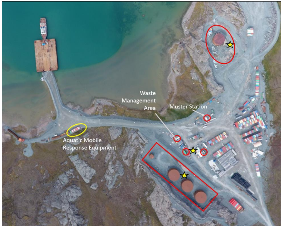
Plate A.1. Roberts Bay Laydown (Note: Red circles are fuel or chemical storage locations, smaller containment locations may vary. Yellow stars [or a yellow circle in the case of the aquatic mobile response spill equipment] indicate default spill kit locations.)
