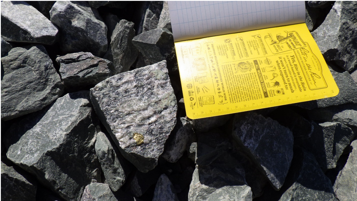
Photo: Sulphides observed at South Dam
