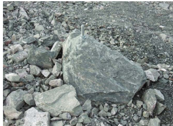
Example of deep settlement points installed in the downstream of the dam.
