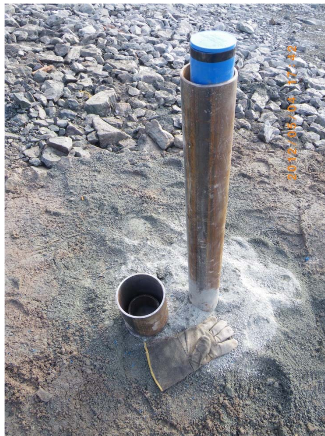
Example of inclinometer protective casing, with and without top cap on.
