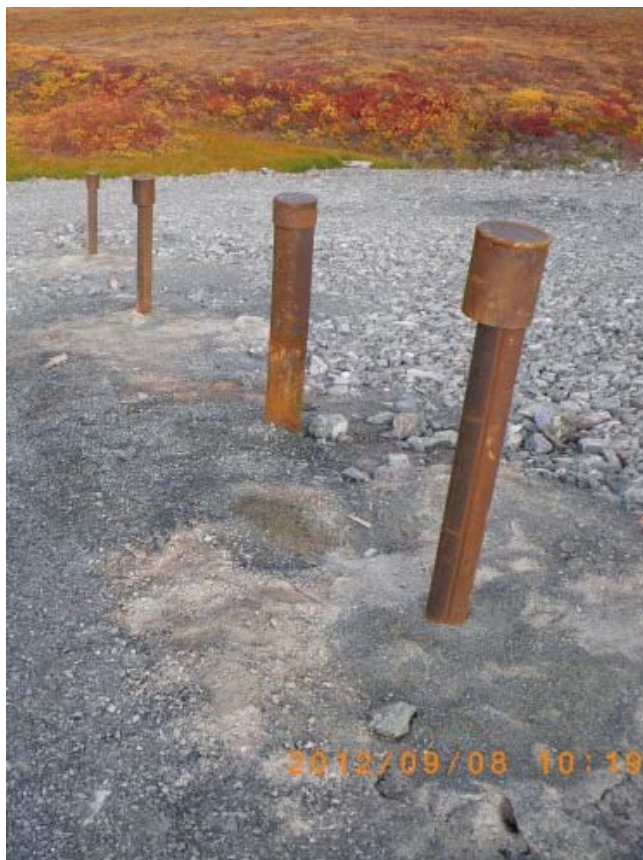
Example of inclinometer protective casing, with and without top cap on.
