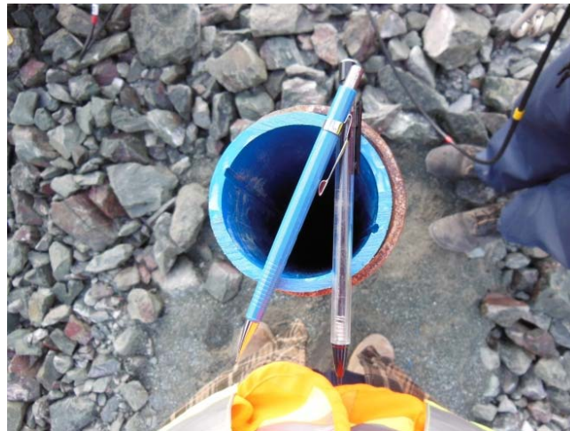
Example of four inner grooves spaced at \sim 90^\circ angles. Note that only one set of grooves is used for the two sets of measurements (i.e. 180^\circ rotation of instrument)
