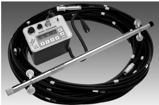
Example of Digitilt Inclinerometer Set-Up
