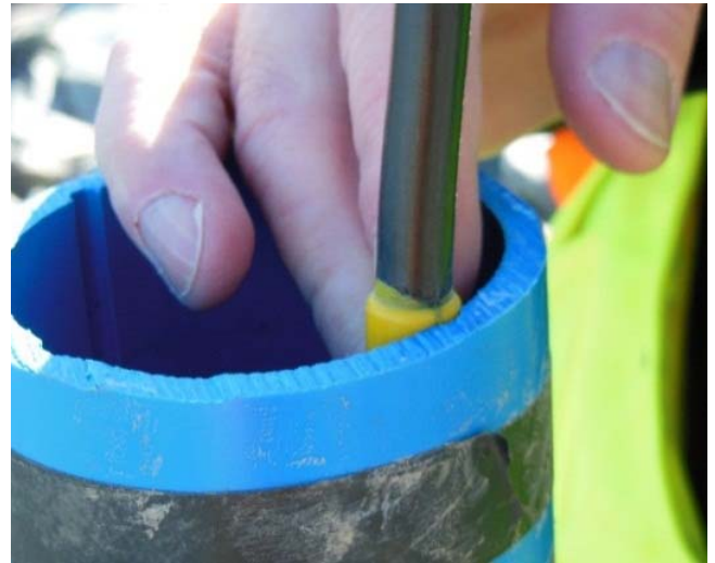
Marker being correctly held and aligned with top of inclinometer casing
