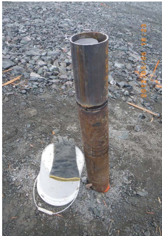
Example of deep settlement points installed in the downstream of the dam.
