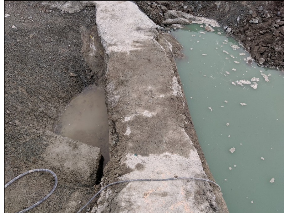
Dye testing plinth 3. July 16. 2019
