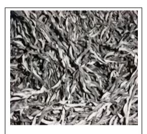
Figure 1: BIONEST ™ media offering a support for microorganisms
