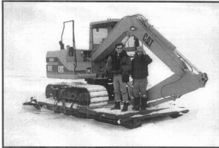
Plate 3-Caterpillar 307 Excavator: A light excavator is required to work within the trench
