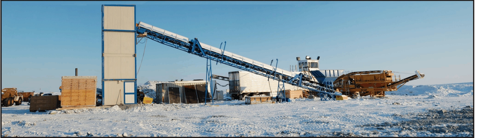
Photograph 2 Crushing Plant and Sample Tower Arrangement
