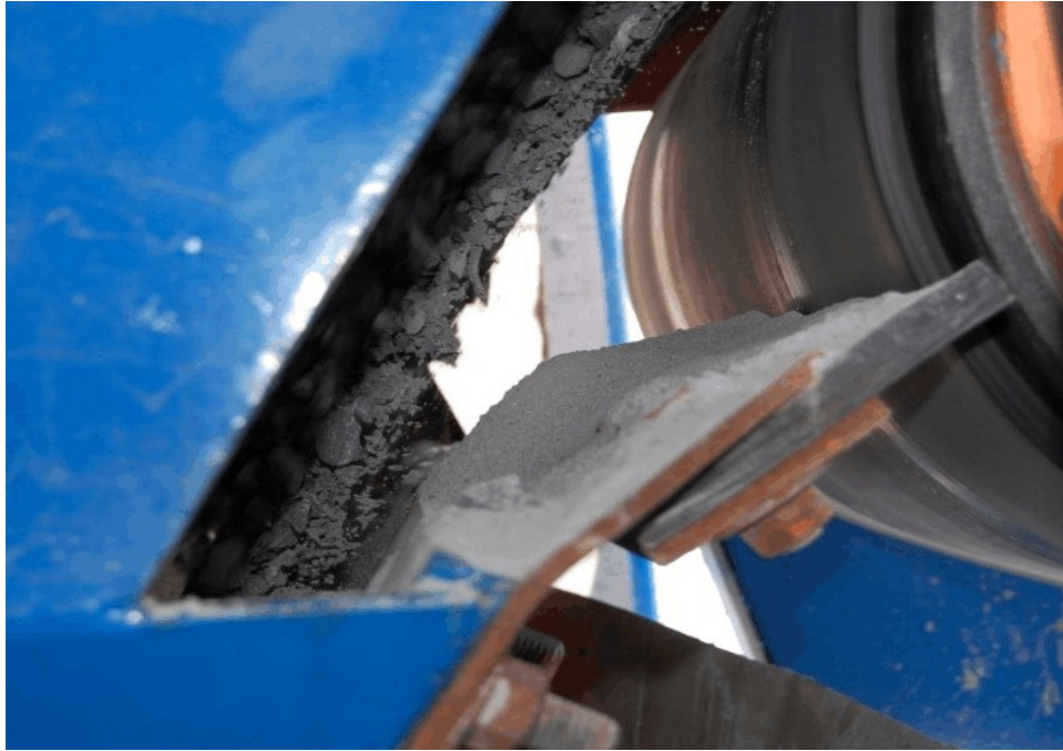
Side view of flow into the sample tower
