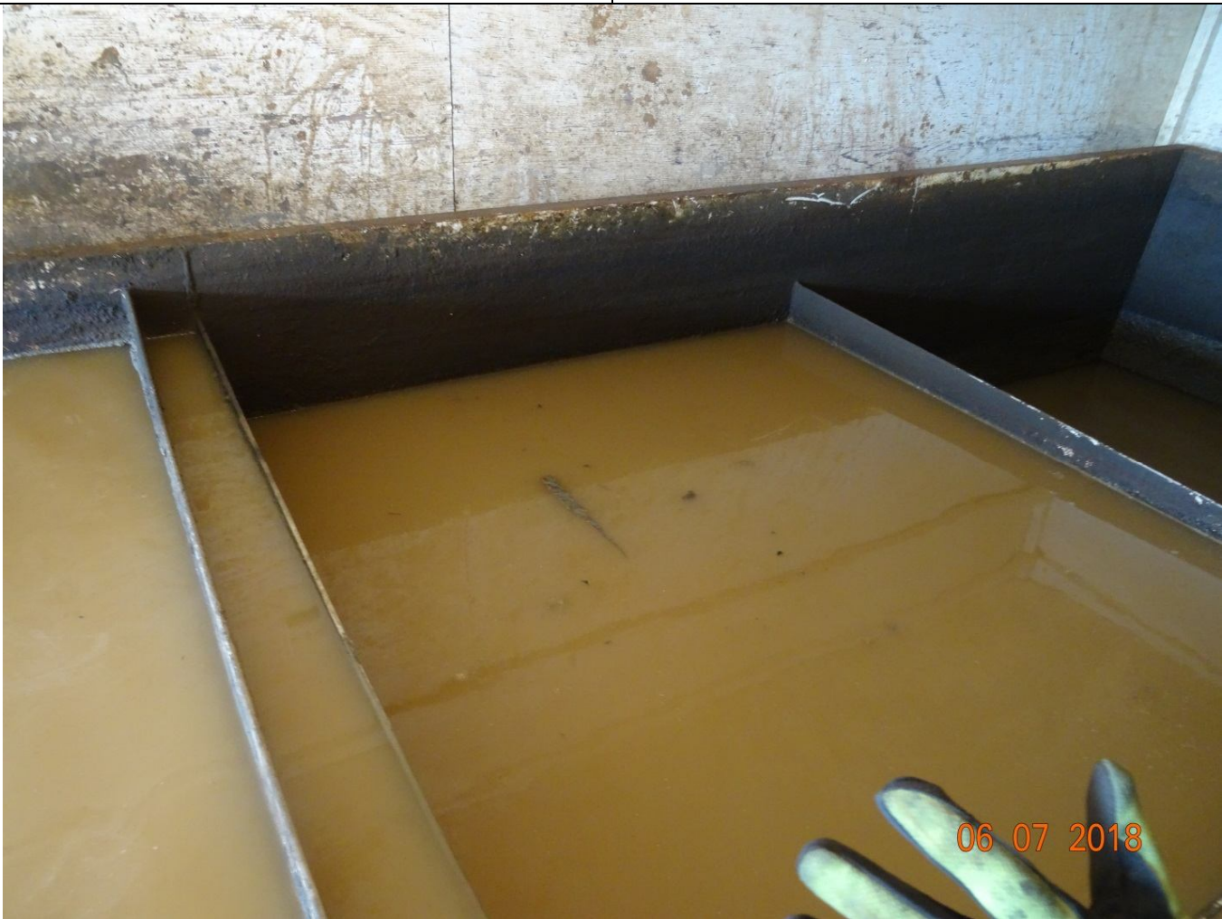
Description: Drill 1: Three stage settling tank with flocculants inside Orbit Garant Drill.
