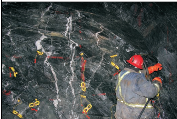
2E: Loading a new face with explosives for blasting
