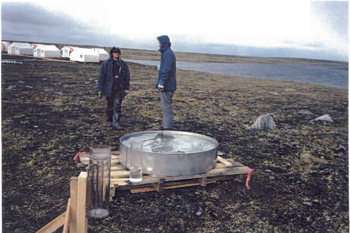
Photo 30. June 24, 1997. Evaporation pan being installed. Note submerged max-min thermometer, stilling well with internal point gauge, graduated cylinder, and post-mounted manual rain gauge.
