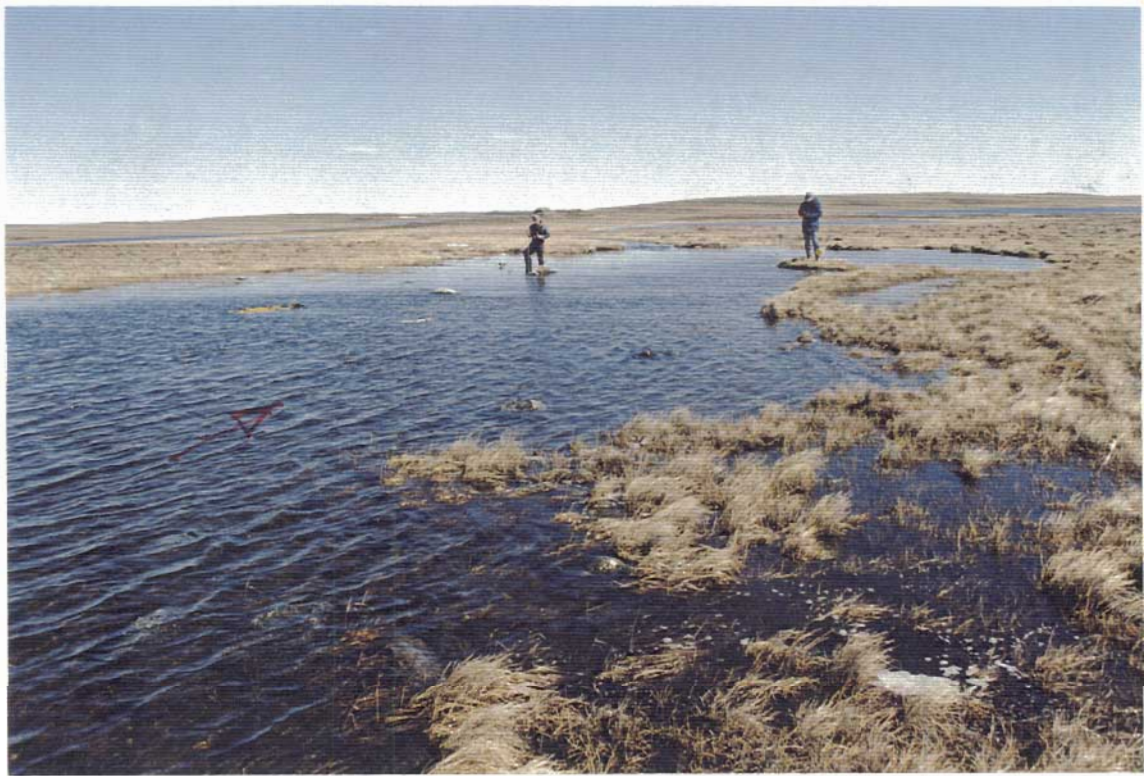
Photo 11. June 12, 1997. Peg Lake outlet looking downstream. Discharge measurement in progress.
