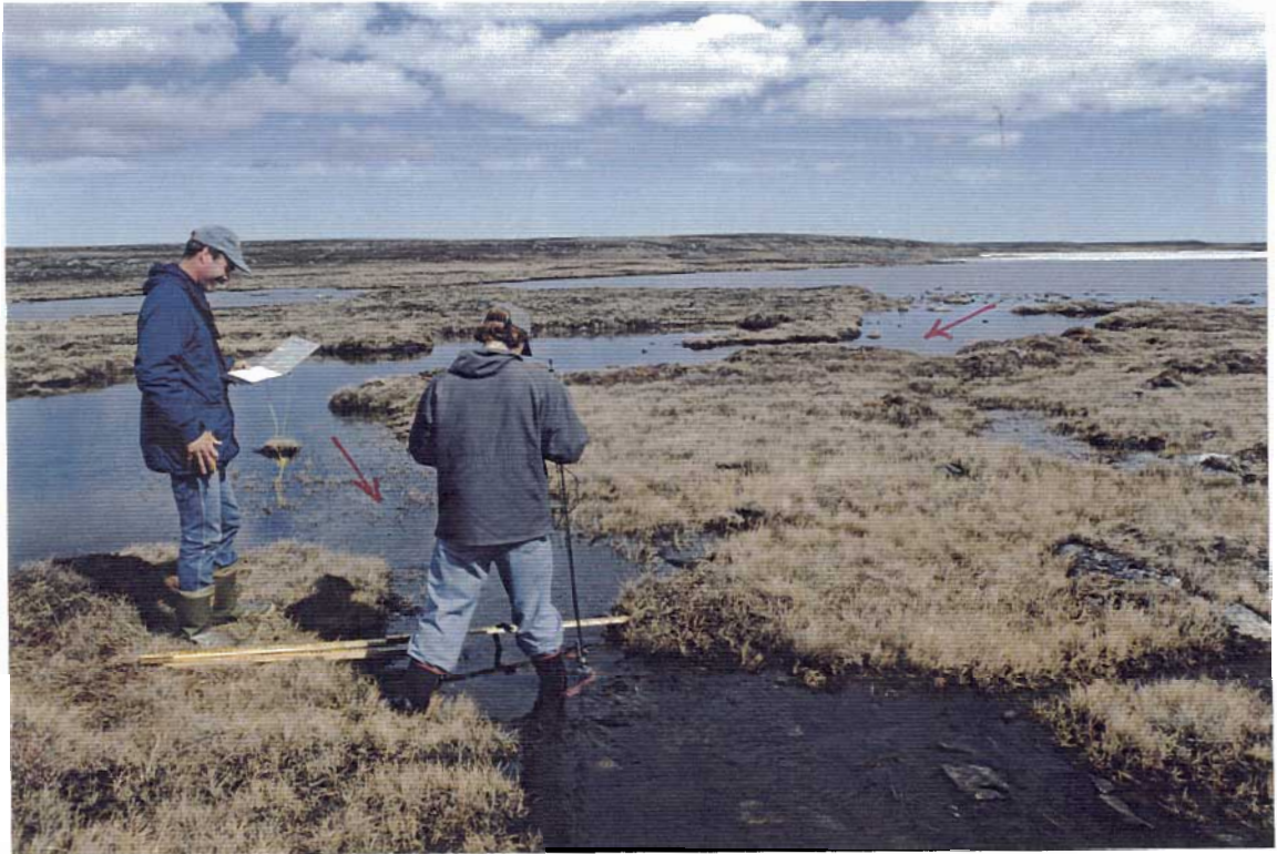
Photo 29. June 12, 1997. Control Lake outlet looking upstream. Discharge measurement in progress.
