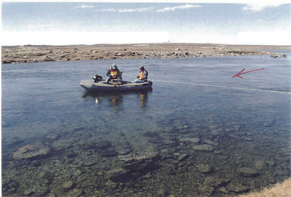
Photo 5. June 12, 1997. Meliadine River near the mouth. Measuring the discharge.
