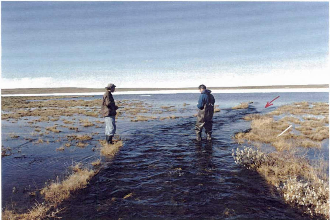
Photo 20. June 10, 1997. Newy Lake outlet looking upstream. Discharge measurement in progress.
