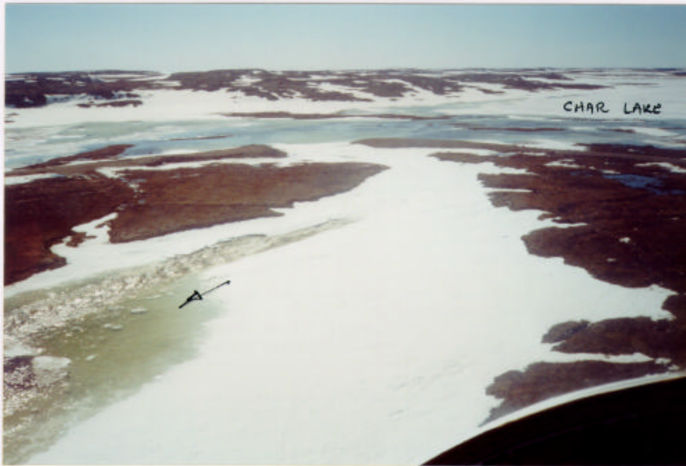
Photo 5: June 13, 2000. Char River looking upstream from vicinity of road crossing. Flow occurs both through and over the snow which fills the channel.
