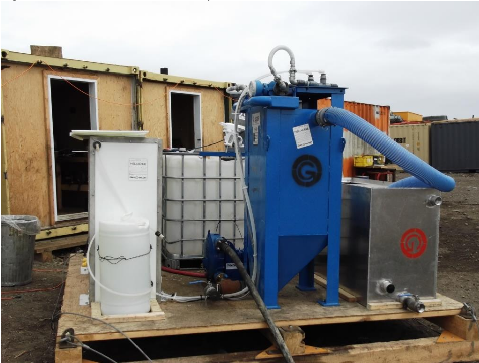
Figure 1, drill water recirculation system
