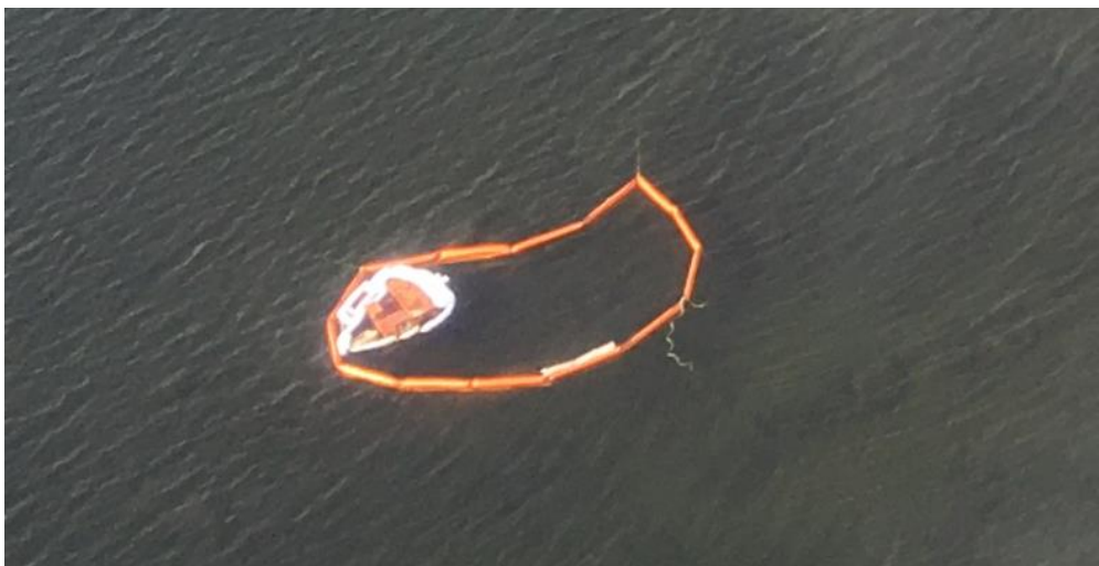
Figure 3. Fuel tank inside containment barrier and absorbent booms
