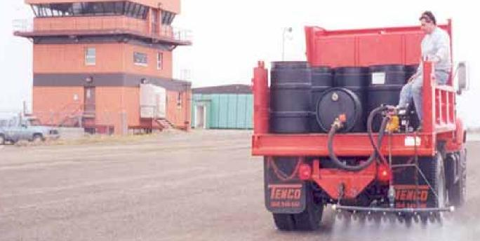
On alpha taxiway beside the apron to evaluate performance and impact on an operational surface. (Curing, stability, crust potential)
