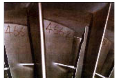
FOD damage to engine blades (below) and wings (above) can be dangerously severe
