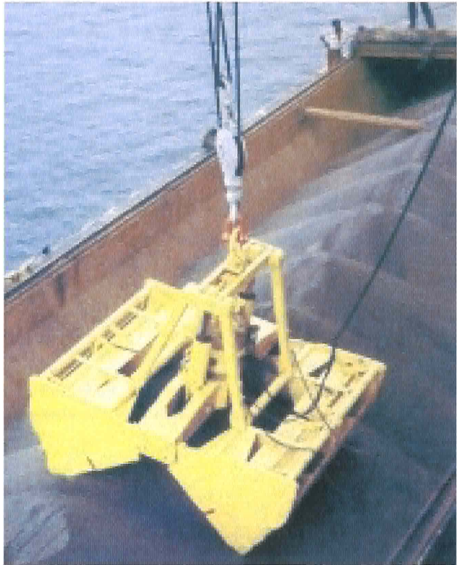
Photo 5 A grab, used by ships to transfer ore from barges to the ship
