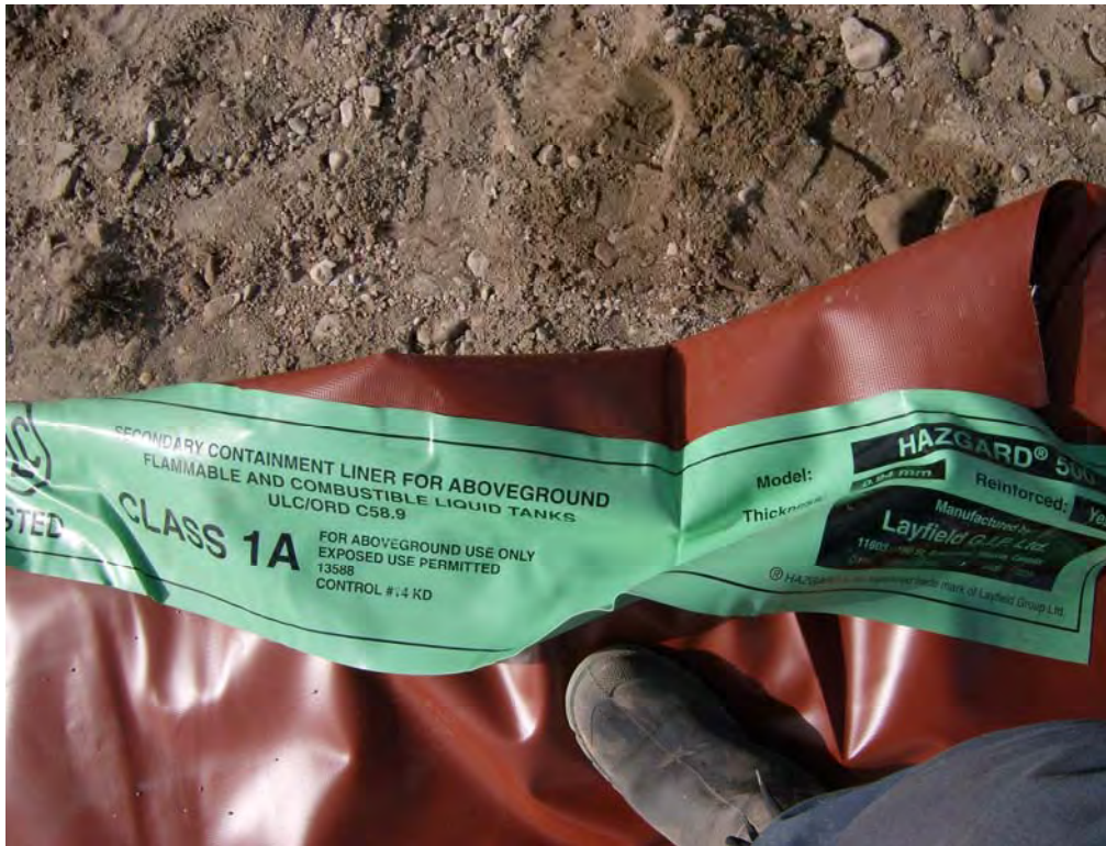
Photo 5: The liner material is shown above.
