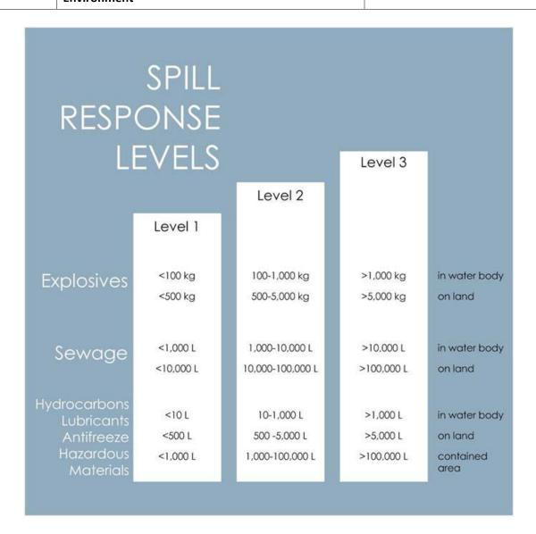
**FIGURE 2-1: SPILL RESPONSE LEVELS**
