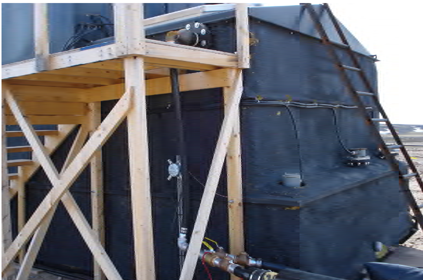
Photo 2: Seprotech N70 RBC Unit, looking closer
