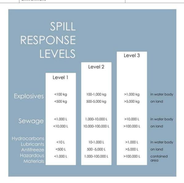
**FIGURE 2-1: SPILL RESPONSE LEVELS**
