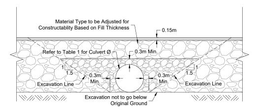
**Typical Cross Section of Single Culvert Crossing**
