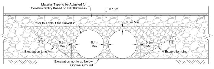
**Typical Cross Section of Double Culvert Crossing**
