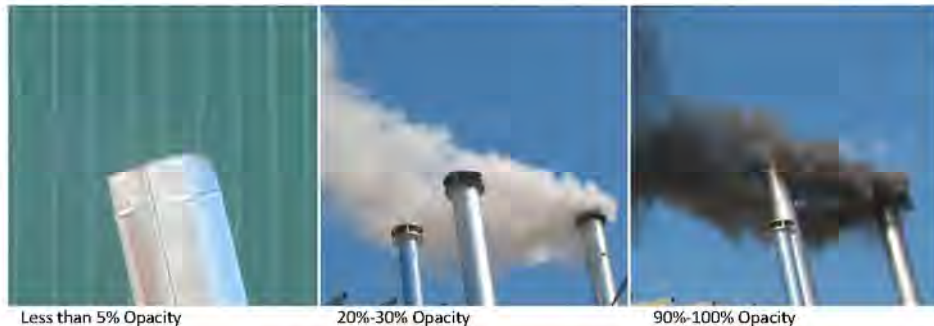
Figure 6 - Examples of Smoke Opacity Ratings
