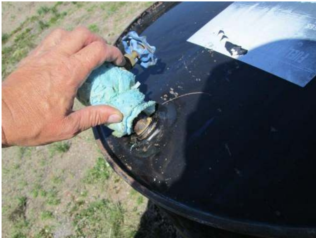
Photo 4: Broken Valve on Fuel Drum
