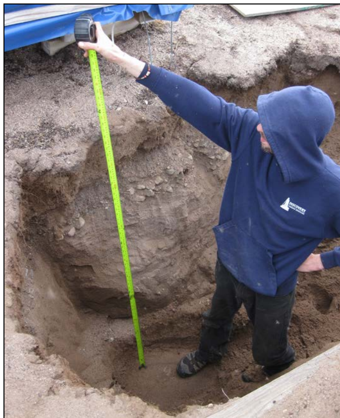
Figure 3: Excavated Pit – 1.4 metres to Frozen Permafrost Layer
