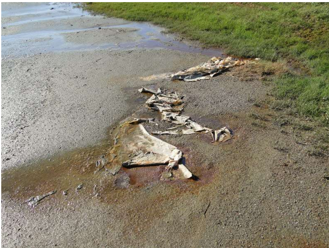
Figure 5. Staining on the shore downhill from waste. Water sampling tested positive for Hexane Extractable Materials.
