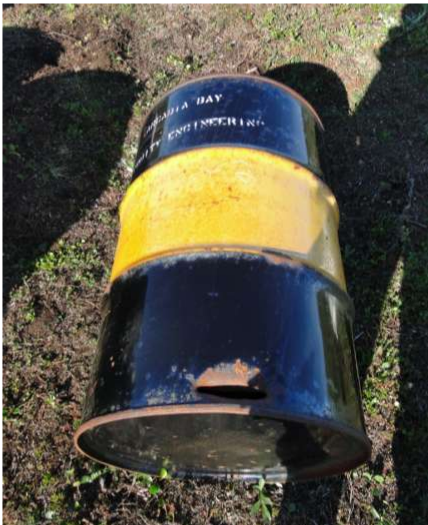
Figure 4. Punctured drum - still half-full of fuel. [117324.2]
