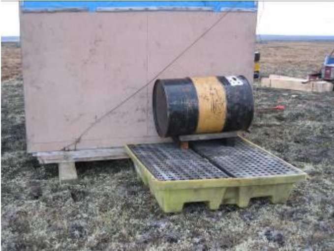
Above: Example of proper secondary containment for diesel fuel at drill site. Below: before and after pictures from a typical diamond drill set up.
