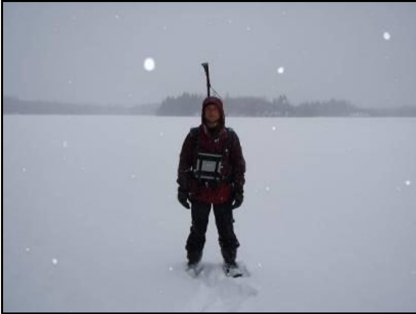
Above: Ground Magnetic surveying by foot using snowshoes in winter.
