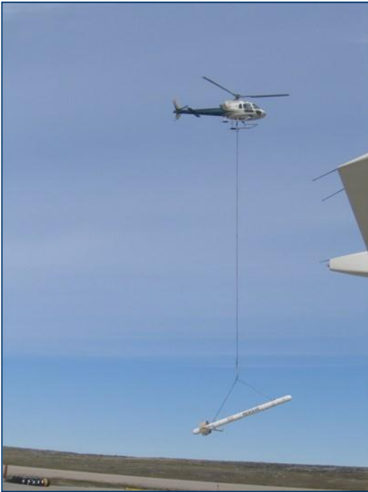
Above: Helicopter based airborne geophysical survey that is towing the sensor.
