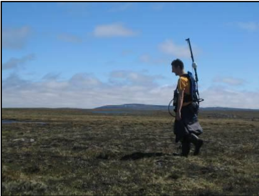
Above: Ground Magnetic surveying by foot in summer.
