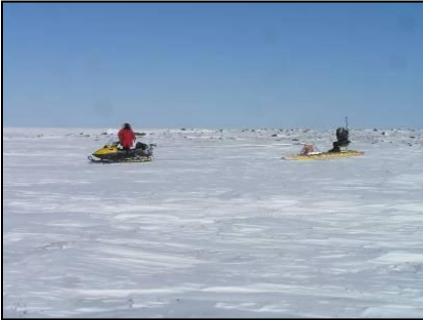
Above: Ground Magnetic surveying by snowmobile in winter season using a snowmobile that tows a sled mounted with the measuring device.
