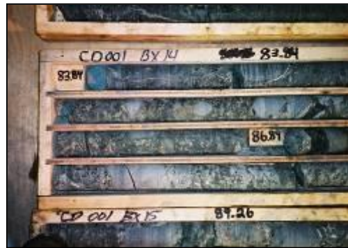
Above: Pictures show examples of drill core of kimberlite. On right drill core is organized in core boxes for proper logging.
