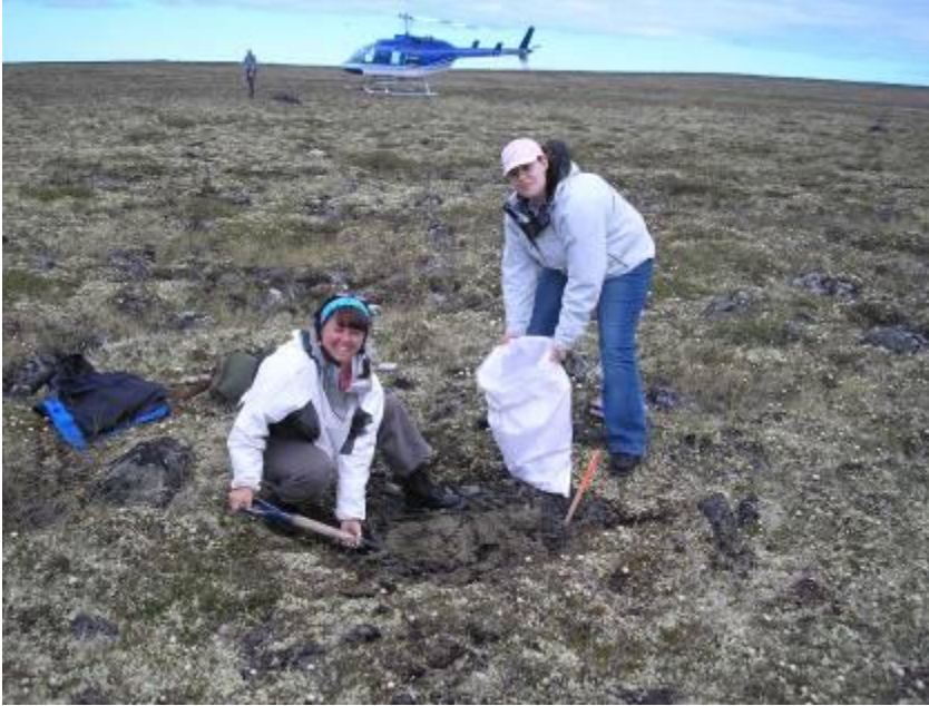
Above: Crew actively collecting till sample. Below: Example of till sample site once collected. Sample bags are shipped off site for analysis.
