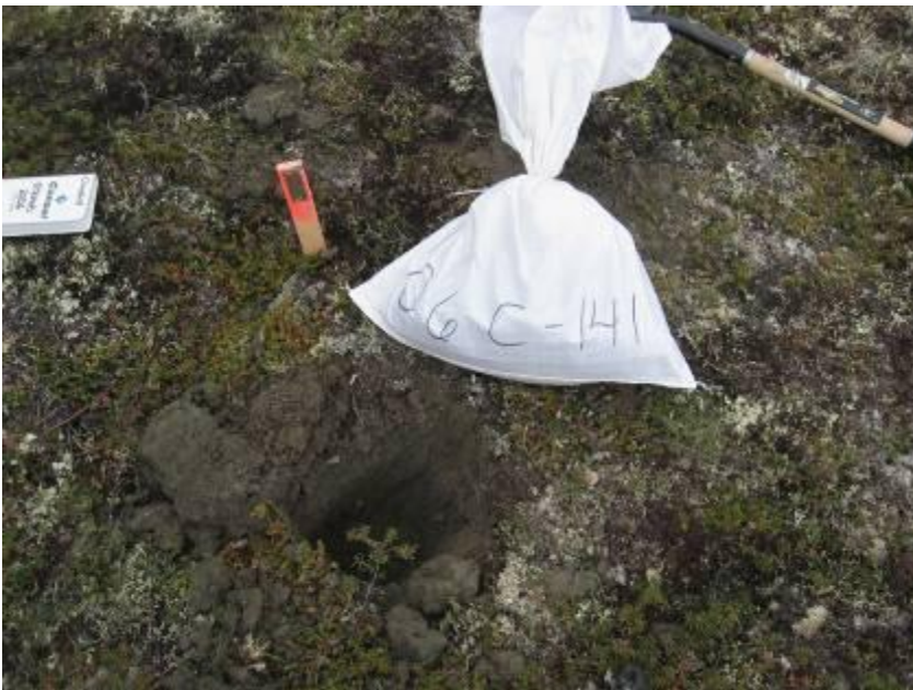
Above: Crew actively collecting till sample. Below: Example of till sample site once collected. Sample bags are shipped off site for analysis.
