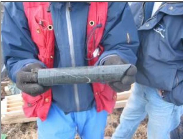
Above: Pictures show examples of drill core of kimberlite. On right drill core is organized in core boxes for proper logging.
