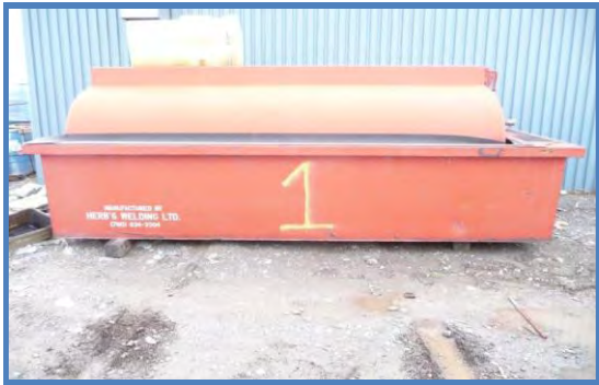
Fuel enviro-tank with spill containment
