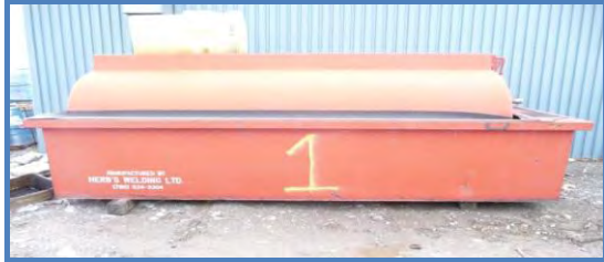
Fuel enviro-tank with spill containment
