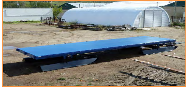
Fuel sleigh that enviro-tank will be secured to
